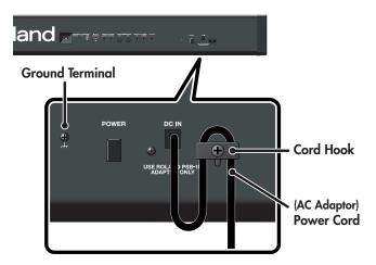
To prevent the inadvertent disruption of power to your unit (should the plug be pulled out accidentally), and to avoid applying undue stress to the AC adaptor jack, anchor the power cord using the cord hook, as shown in the illustration. Even if the cord is fastened, strong tension applied to the cord may cause it to be damaged or broken. Be careful not to pull the cord accidentally, or to apply strong pressure to it.
